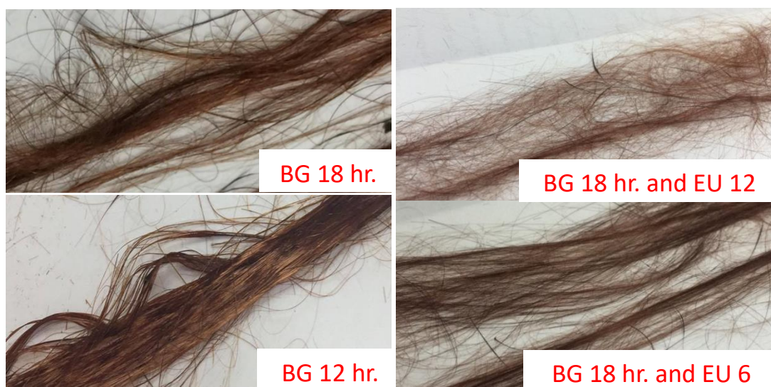
Figure 3. Organosolv lignin fibers
